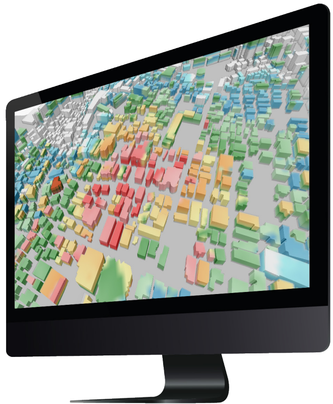
Figure 3. An example of a 3D-analysis of LTE Reference Signal Received Power from one site in an urban area, displayed in Planet. High signal levels are in red, low signal levels are in blue.
