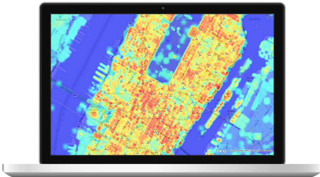
Figure 4. A total traffic map for Manhattan in Planet. Social media traffic, carried traffic and high-resolution geodata combined to make an accurate traffic model. Showing areas with the high (red) and low (blue) traffic demand
