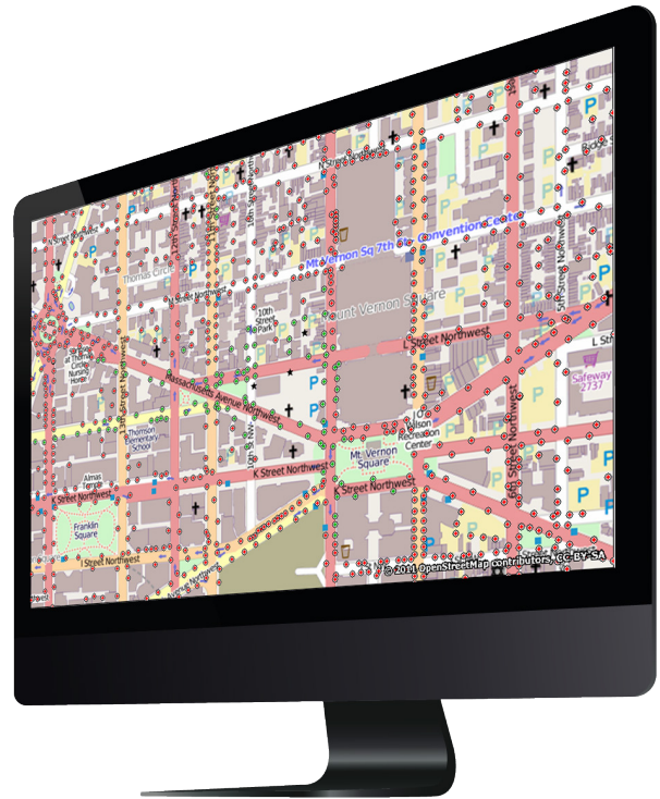
Figure 6. A database with street lights in Washington, D.C. has been analyzed for backhaul connectivity in Planet. The street lights with line-of-sight to access points (green dots) are potential locations for small cells. The street lights lacking line-of-sight (red dots) are not candidates for conventional microwave links areas.
